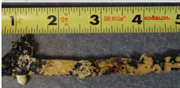
Fig.2 Close up of another field sample of hard ,glassy off ratio foam with some adhesive ability but not much
