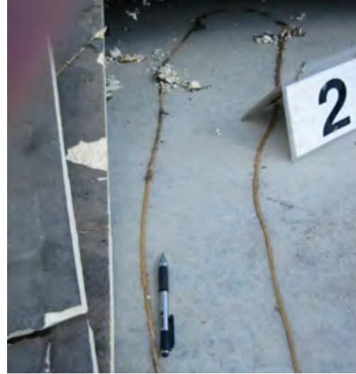
Fig.1 Hard glassy, off ratio low rise foam; has little adhesive strength, no foam expansion.
